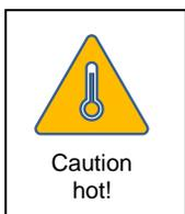
Under normal operating conditions the surface of the device can become very hot! Under the maximum operating conditions, the surface temperature can exceed 350°C. After shutting off or, if necessary, shutting down the boiler, wait until the temperature has normalized to room level. To avoid the risk of burns and scalds, always use PPE including safety goggles!
